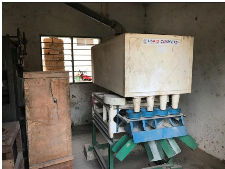
Plate 13: Rice grading machine at Mang'ula 'A' warehouse facility
